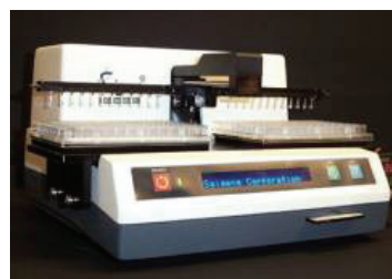
Figure 3. Automated processor (Saigene) for sandwich hybridisation assay
