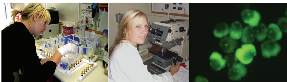
Figure 1. Filtration rig (left); epifluorescent microscope (middle) and view of positive assay using fluorescein-tagged oligonucleotide species-specific probe targeted at Karenina mikimoto (right).
