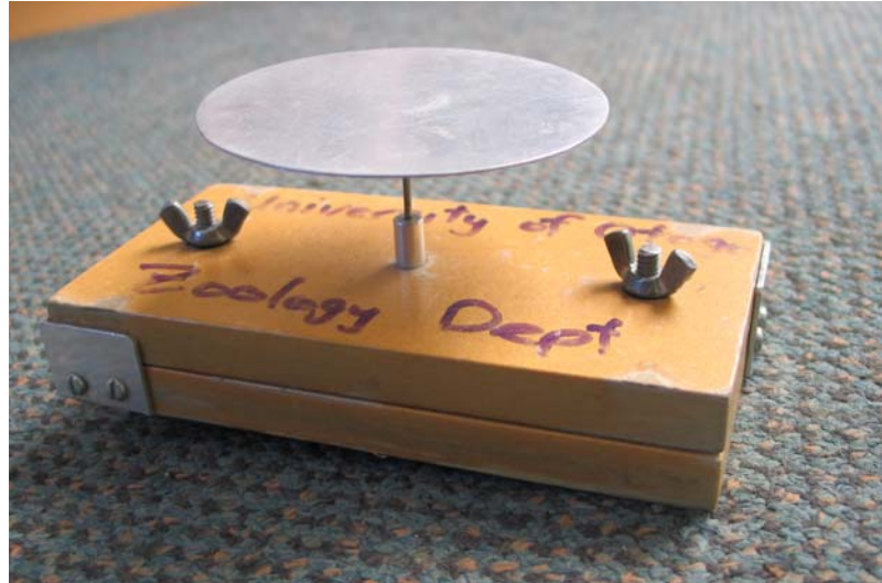
Figure 2 The penetrometer used to measure leaf toughness
